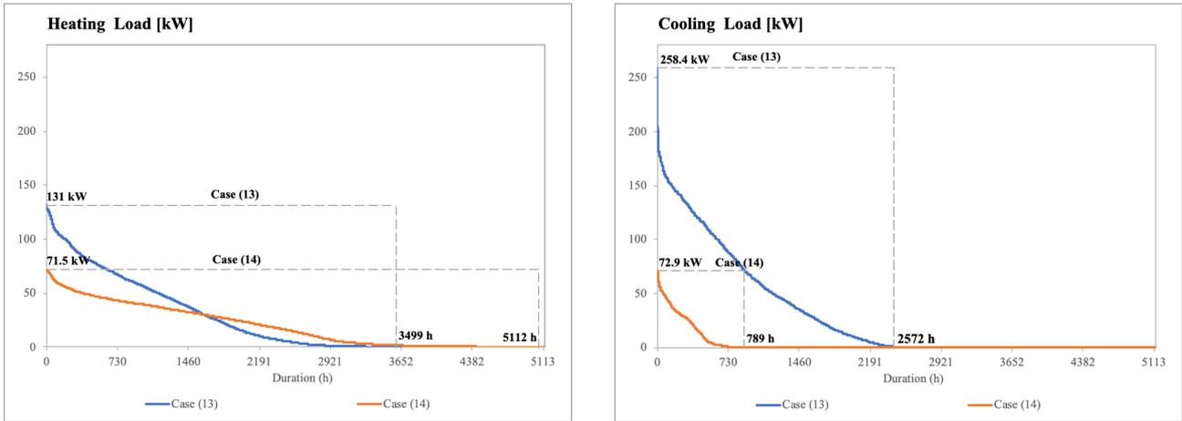
**Fig. 8.** Heating and cooling load duration curves for the cases of (13) and (14)
